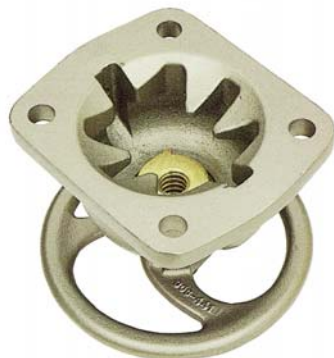
PVDF corrosion resistant coated bonnet shows the molded-in fingers utilized to support the diaphragm in the open position.
